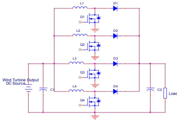
Fig. 3. Schematic diagram of 4-phase interleaved boost converter.
