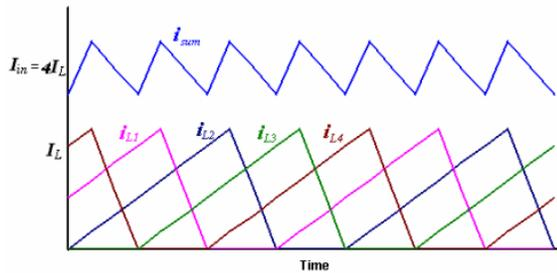
Fig. 4. Input current and inductor current waveforms of a boost converter operating in DCM.
