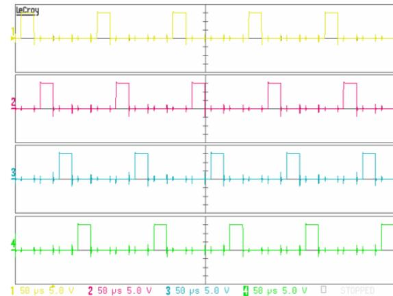
Fig. 9. Gate drive signal waveforms of 4 phases.
