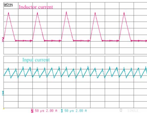
Fig. 11. One phase inductor current vs input current.
