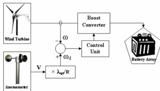
Fig. 1. The block diagram of a wind turbine control system.
